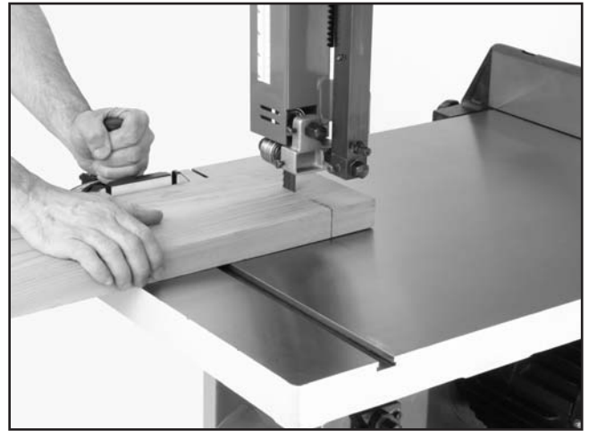
Figure 32. Crosscutting with the miter gauge.
